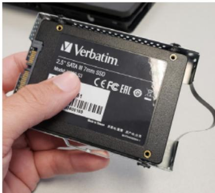
3.8 The gold connectors should be visible and inserted first into the drive bay. Slide the drive bracket with SSD back into the drive bay of the PS4™. Make sure to slide it all the way in to ensure the connectors inside line up.
