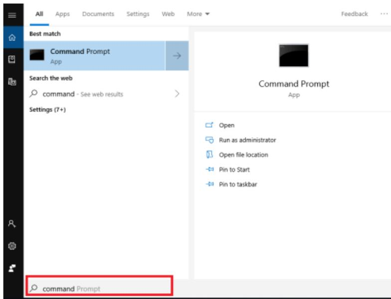
5.10.2 Type "list disk" (without quotations) and hit enter. Record the disk number. Then type "select disk X" (without quotations) where X is the disk number. Make sure to choose the PS4™ HDD and not your operating system HDD. Hit enter. Type "clean" (without quotations). Hit enter. A prompt will notify that the disk has been cleaned and is ready for a fresh formatting. Close the Command Prompt program.
