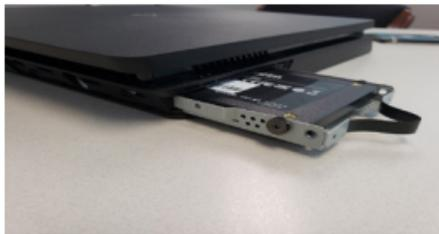
3.9 Screw the single silver screw into the back of the PS4™ housing.
