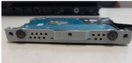
3.6 Remove the HDD from the drive bracket and carefully set aside.
