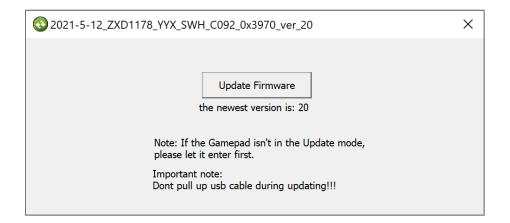
**Step 5:** While continuing to hold the joystick down, click "Update Firmware." Once the update is complete, the pop-up message "Update Success!" will appear (example shown below). You can now release the joystick and disconnect the controller from the computer.
